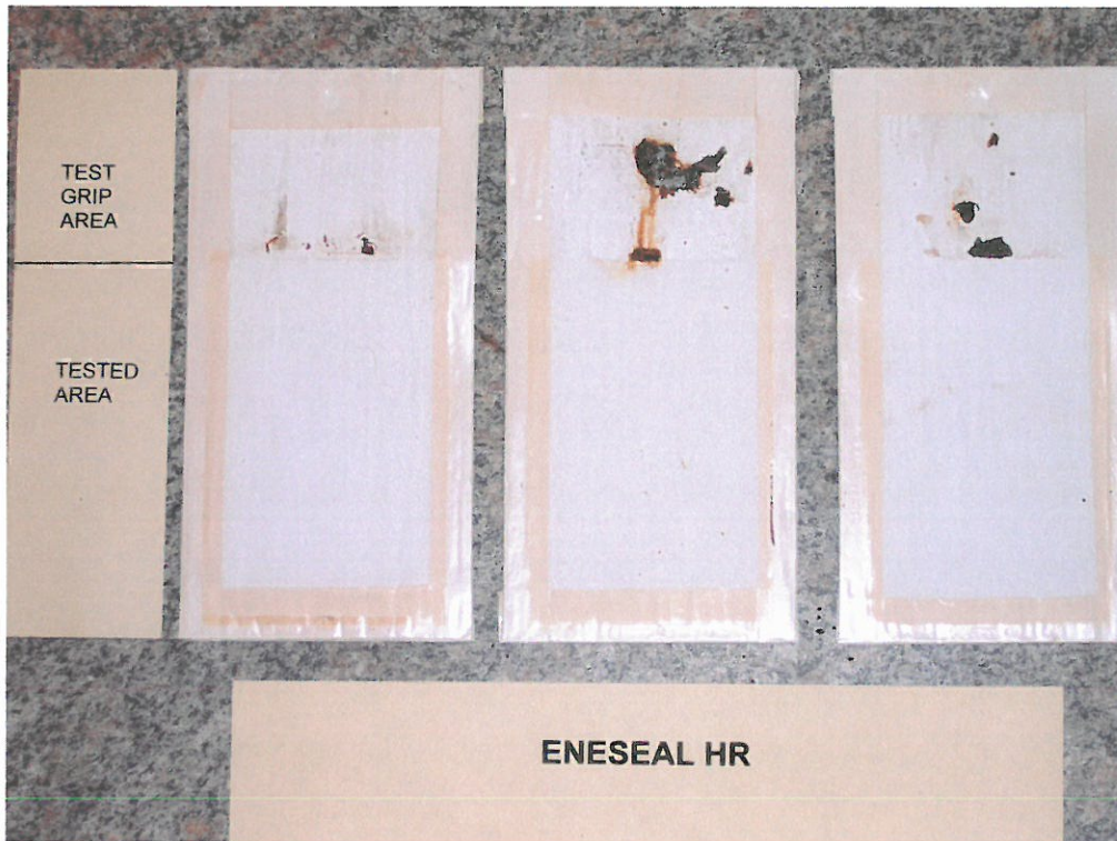
Photo 1 – QUV Weather-O-Meter ENESEAL HR panels after 1000 hours
